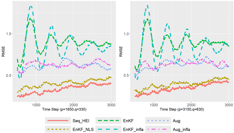
FIGURE 6 RMSE of the data assimilation results by six different methods, Seq_HEI (proposed), EnKF_NLS, EnKF, EnKF_infla, Aug, and Aug_infla, for the shallow water model with (T, n) = (3000, 25) .
